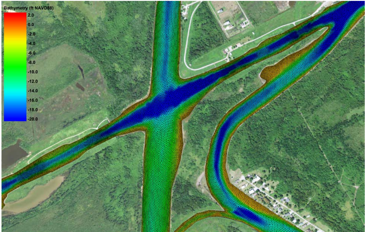
Figure 38 AdH mesh for Open-Channel Alternative
