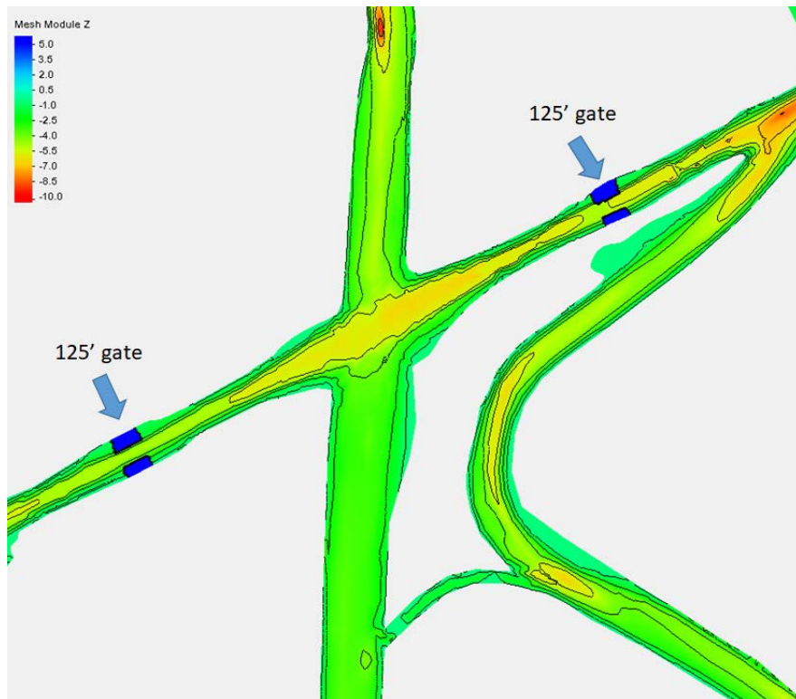
Figure 63 . AdH mesh bathymetry for with-project condition AdH mesh with 125ft single gate system
