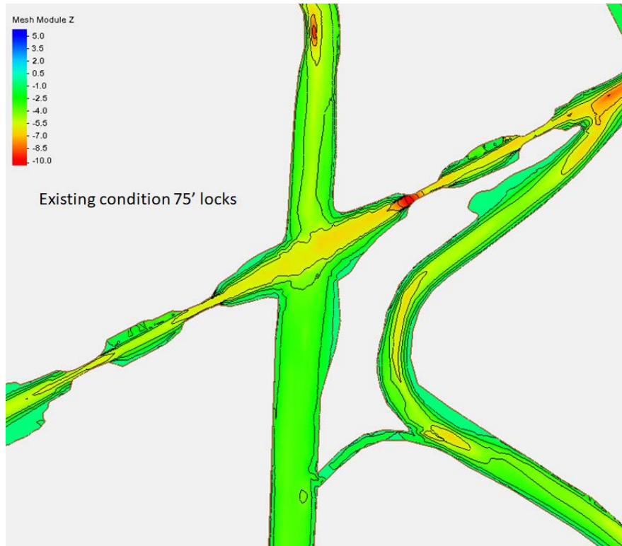
Figure 62 AdH mesh bathymetry for existing condition AdH mesh with 75ft lock system
