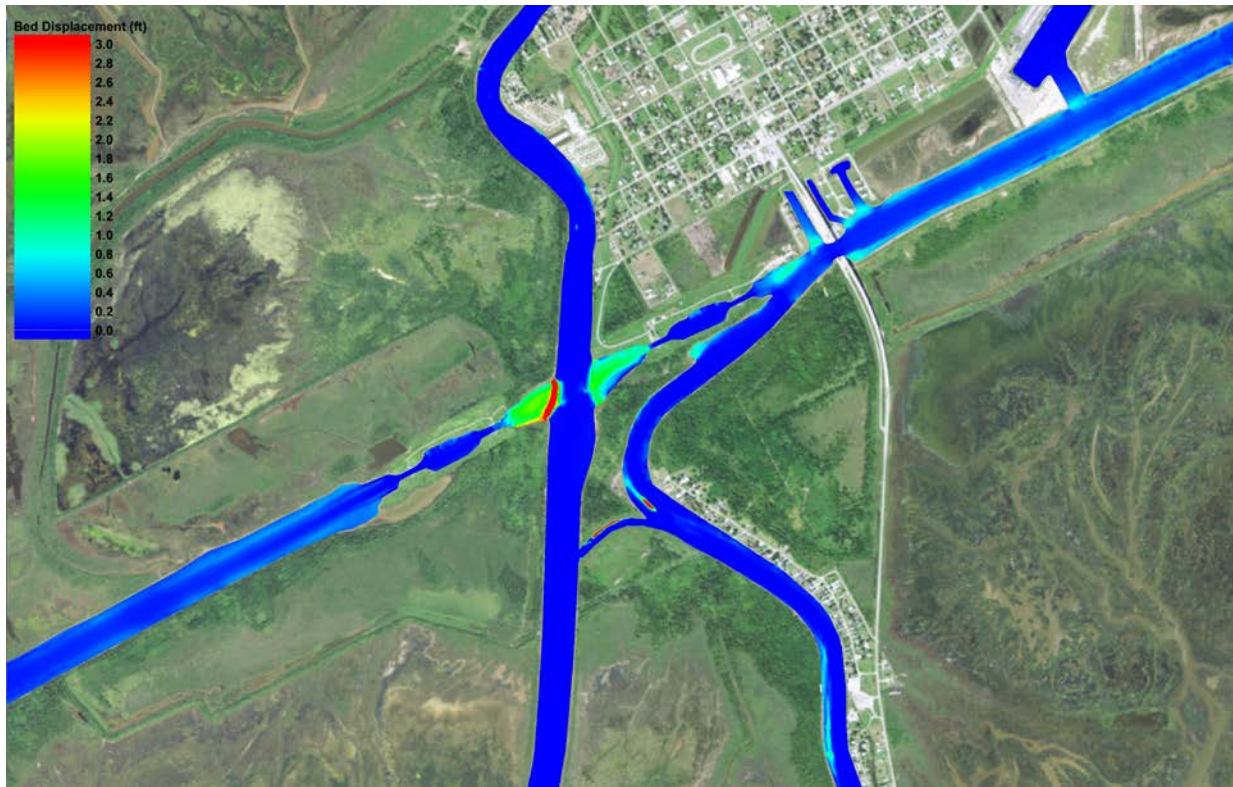
Figure 49 Bed Change at end of 2016 Simulation for Existing Conditions
